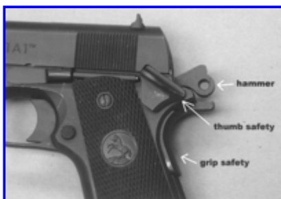
Fig. 2C. —Photographs of 1991 A-1.45 caliber semiautomatic pistol (Colt's Manufacturing, Hartford, CT). Hammer, thumb safety, and grip safety of gun are shown. Gun is in cocked and locked position with hammer cocked and thumb safety turned on to prevent hammer from striking firing pin. This is condition in which gun was recovered from magnet.
